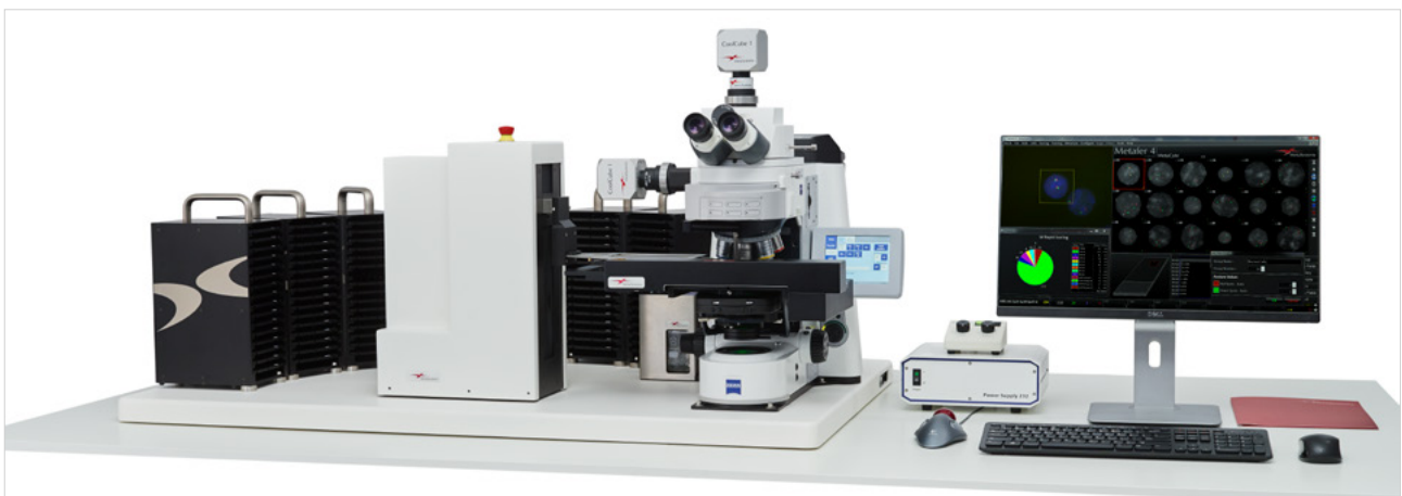
Figure 1 Metafer from MetaSystems is a versatile, automated microscopic image-capture and image-analysis platform. Today's Metafer systems are based on continuous development and diversification that has been carried out over a period of more than 30 years.
